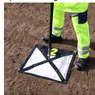
Img31: ground control point
